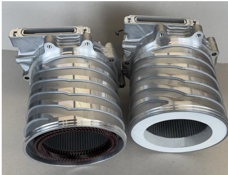
Example hairpin motor unencapsulated and encapsulated
